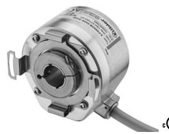
The optical Sendix F5888 multiturn encoder in the Motor-Line version stands out particularly because of its reduced overall depth of only 43 mm with a through hollow shaft up to 15 mm.
