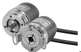
The Sendix F36 multiturn with the patented Intelligent Scan Technology™ is an optical multiturn encoder in miniature format, without gears and with 100% insensitivity to magnetic fields.
